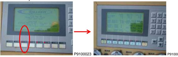
4. Press the F3 Toggle mode switch from standby to run mode. All programing and running job is done in run mode. (no data will be recorded or monitored by TMV while in standby mode)
