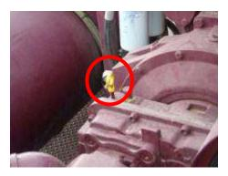
5. **Cleanout fluid tanks:** Check the cleanout tank levels by removing the cleanout tank cap and visually inspecting the fluid level. Cleanout fluid level must be at approximately the bottom of the fill spout. If fluid is low, contact a mechanic or supervisor for the correct fluid and fill as specified.
